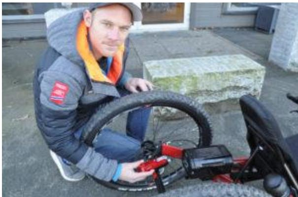
*LIMITED PRESSURE: SMART BRAKE requires only a small push on the handle to slow down. The transfer is done wirelessly to the disc brakes of the recumbent bike. The solution also acts as a parking brake, explains Henrik Karlstad.*
